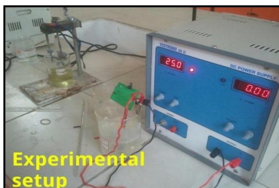
Fig 1: Experimental set up of anodizing process
